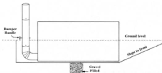
Mount the elbow and pipe to stick straight up. (See sketch "D"). Fasten the elbow to the collar with two of the metal screws and fasten the pipe together with two screws at each joint.
